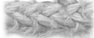
Rope must be replaced
