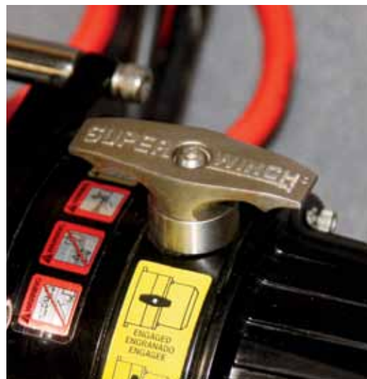
Our panel of judges gave mixed reviews on the unit's unique stainless steel T-handle clutch lever.
