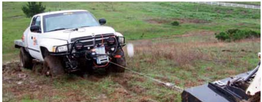
The Warn model was faster than the rest but demanded more electrical energy than our test arrangement could supply, so it depleted the battery and ceased forward momentum halfway up the hill.
