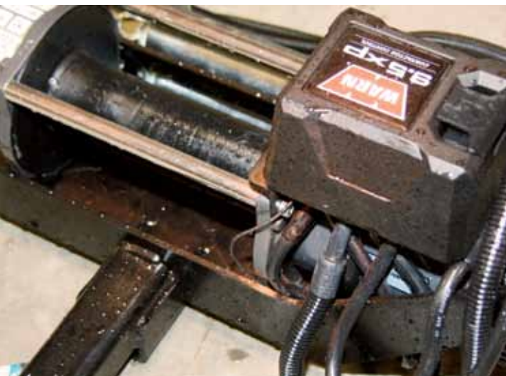
◀ This photo shows the thin film of Aeroshell #17 lubricant left behind after running the unit under water for a ten-minute period.
