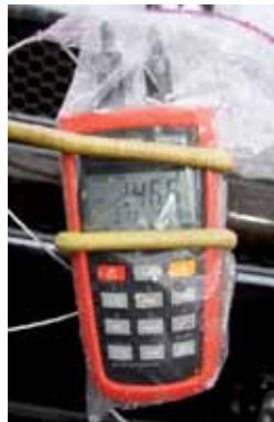
◀ This is the Omega digital temperature recorder we used for the shootout. The two-channel unit displays the temperature of two wired thermal couplers. We attached one thermal coupler to the exterior of the winch motor and another to the gear case on the opposite side.
