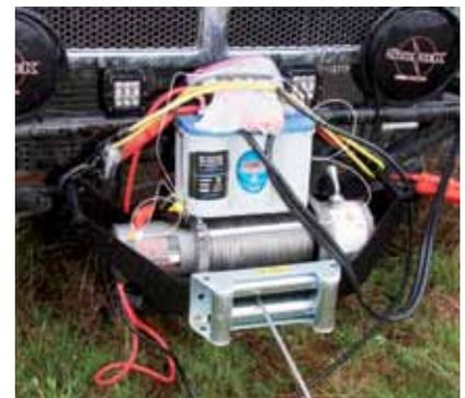
▶ Each winch was tested with a fully charged Optima BlueTop deep-cycle battery. The batteries were wired into the vehicle's charging system using Warn's quick-disconnect harnesses. An isolation switch ensured that the existing batteries installed in the truck would not skew our results. The Premier Power Welder alternator supplied each test battery with 195 amps of charging power.
