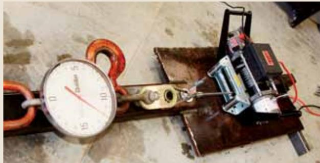
while the load cell was affixed to the other end. The system was massive and could only be moved using a forklift. We used a 10-foot section of ½-inch steel cable to ensure that cable stretch or breakage would not be an issue. The arrangement would allow each winch to reach its maximum pulling power or stall point, while the gauge recorded the maximum pound rating. As you might expect, many of the winches did not survive this torture test.
